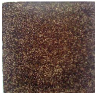
Plate1: Sawdust-palm kernel shell based particleboard Source: Fono-Tamo et al. [28]
