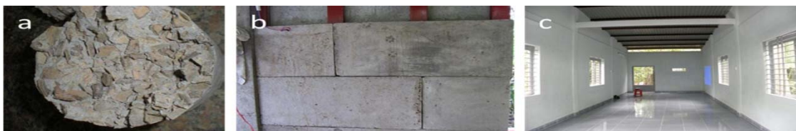
Plate 1. Coconut Reinforced Concretes: a) a concrete block, b) the concrete panels and c) the house built from them
