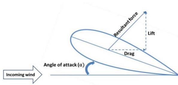
Figure 1: Drag and Lift components of the aerodynamic force (10)
