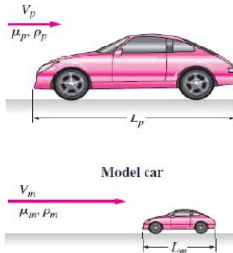
Figure. 13: Showing model of a car and its prototype (Geometric similarity between a Prototype car of length  $L_p$  and a model car of length  $L_m$ ). (Mdp.eng.cam.ac.uk)
