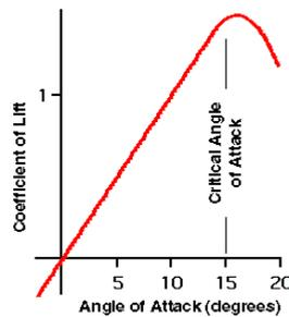
Figure 2: Curve showing relationship between AOA and coefficient of lift (Skybrary.aero)
