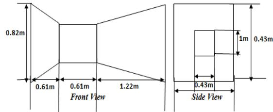
Figure 4: Schematic diagram of the designed wind tunnel
