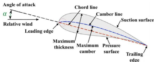
Figure 3: Diagram showing a detailed airfoil [11]
