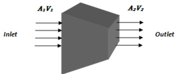
Figure 7: Diagram showing fluid flow across the wind tunnel contraction cone
