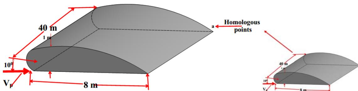
Figure.12: Geometric Similarity in Model Testing (Mdp.eng.cam.ac.uk)
