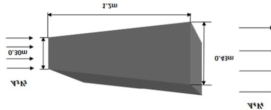
Figure 10: Diagram showing a section of the diffuser assembly
