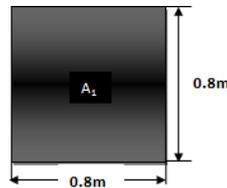
Figure 5: Entrance section of the contraction cone
